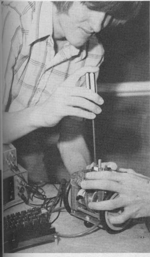
Photo 7: The printed circuit board, shown attached to the Turtle's motor drive housing.
